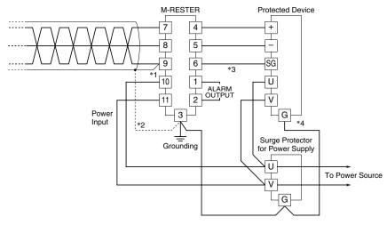
\*1. No need of this part of the wiring if the cable has no shield.
