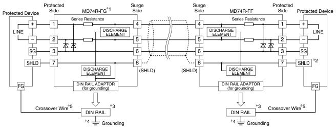
\*1. Choose the MD74R-FG when the shield wire is to be grounded.
