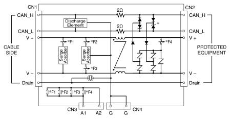
\*DO NOT CONNECT the communication line across CAN\_H and CAN\_L. Such a wrong connection may destroy diodes, or result in a network malfunction caused by a power line voltage decrease.
