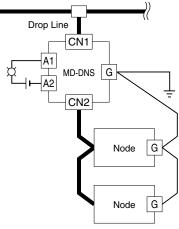
Max. 4 MD-DNM/-DNS can be connected on the single network.
