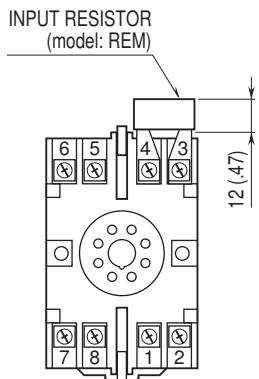
Input shunt resistor attached
