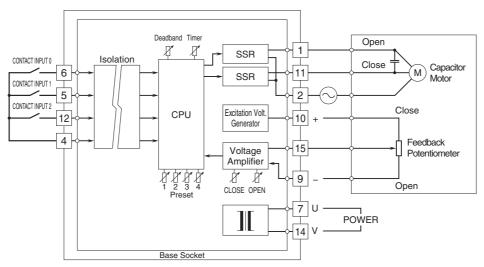
Note: Note that when limit switches inserted in motor wiring, the making/breaking may cause stress on the SSRs.
