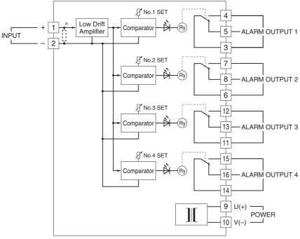
\*Input shunt resistor incorporated for current input.
