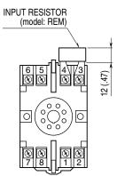
Input shunt resistor attached for current input.
