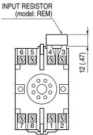
Input shunt resistor attached for current input.
