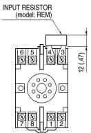
Input shunt resistor attached for current input.
