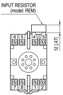
Input shunt resistor attached for current input.
