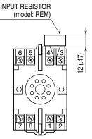
Input shunt resistor attached for current input.
