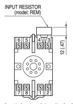
Input shunt resistor attached for current input.
