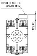
Input shunt resistor attached for current input.
