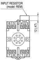
Input shunt resistor attached for current input.
