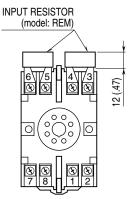
Input shunt resistor attached for current input.
