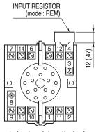
Input shunt resistor attached for current input.
