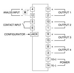
\*Input shunt resistor attached for current input.
