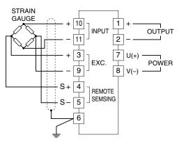
Close across the terminal 3 - 4 and 5 - 9 when the remote sensing is not used.
