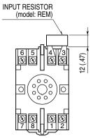
Input shunt resistor attached for current input.
