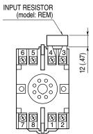
Input shunt resistor attached for current input.
