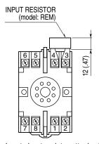
Input shunt resistor attached for current input.
