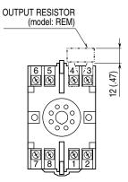
Use output shunt resistor for voltage output.
