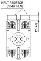
Input shunt resistor attached for current input.
