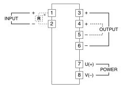
\*Input shunt resistor attached for current input.
