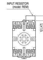
Input shunt resistor attached for current input.
