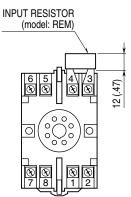
Input shunt resistor attached for current input.
