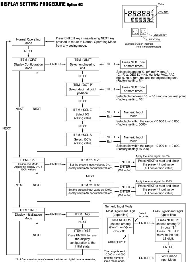
AD conversion value' means the internal digital data representing the input signal, which is computed to a percentage. It is not a % or engineering unit value.
