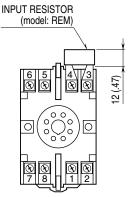
Input shunt resistor attached for current input.
