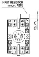
Input shunt resistor attached for current input.
