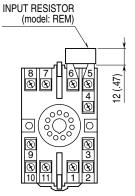
Input shunt resistor attached for current input.
