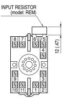
Input shunt resistor attached for current input.
