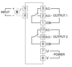
\*Input shunt resistor attached for current input.
