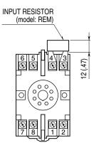
Input shunt resistor attached for current input.
