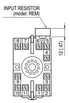
Input shunt resistor attached for current input.
