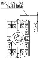
Input shunt resistor attached for current input.
