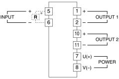
\*Input shunt resistor attached for current input.
