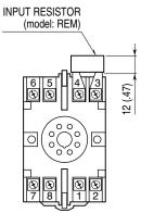
Input shunt resistor attached for current input.
