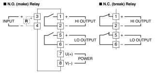
\*Input shunt resistor attached for current input.
