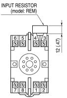
Input shunt resistor attached for current input.
