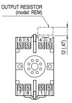
Use output shunt resistor for voltage output.
