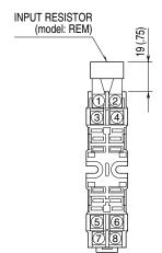
Input shunt resistor attached for current input.
