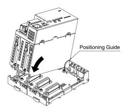
3) Tighten the base fixing screw with a screw driver (stem length: 70 mm/2.76" or more) (torque 0.5 N·m)
