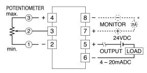
\*DC ammeter's internal resistance 10 ohms max.
