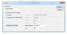
Specify the IP address (Station address) and Service port (Standard Modbus TCP port number is '502').
