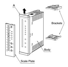
Pull up the part 'A' when replacing the scale plate.
