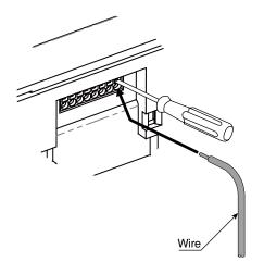
3) Pull out the minus screwdriver to fix wire(s).
