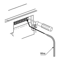
3) Pull out the minus screwdriver to fix wire(s).
