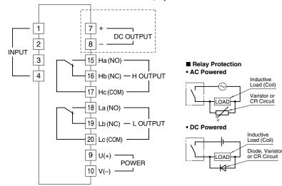
Note: The section enclosed by broken line is only with DC output option.
