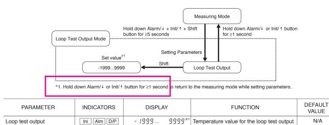
Loopt test output: Pressing [Shift] button switches the signal to increase (Max ON) or decrease (Min ON), and then pressing [Up] button controls it toward the desired output value.
