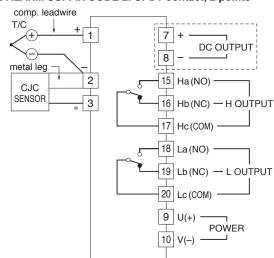
\*DO NOT loosen the screw of the terminal 3. Loosen only the terminals 1 – 2 when connecting extension wires. Note: The section enclosed by broken line is only with DC output option.
