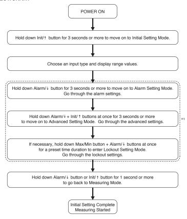
\*1. Optional settings for parameters in a broken-line section. Alarm Setting Mode is locked with no-alarm-output type.
