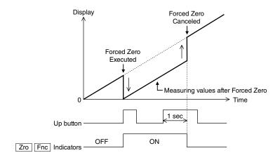
Press Up button to shift the present display value to 0 and to continue measuring in reference to this point.
