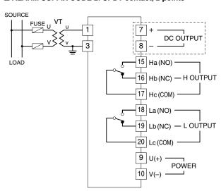
Note: The section enclosed by broken line is only with DC output option.
