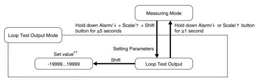
\*1. Hold down Alarm/↓ or Scale/↑ button for ≥1 second to return to the measuring mode while setting parameters.
