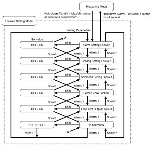
${\rm *1.\ Preset\ time\ can\ be\ specified\ with\ "Transition\ Time\ to\ Lockout\ Setting\ Mode"\ in\ Advanced\ Setting\ Mode.}$
