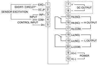
\*Close across the terminals for open collector or mechanical contact. Refer to the figure below.
