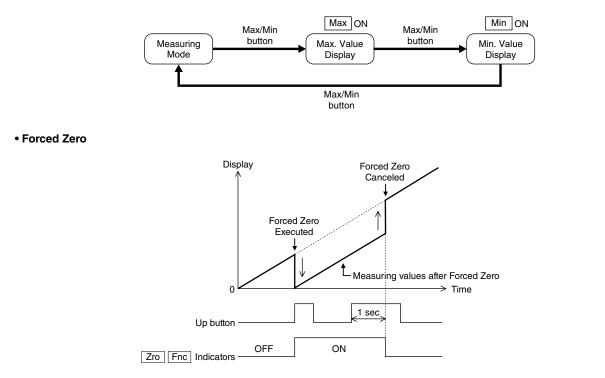
Press Up button to shift the present display value to 0 and to continue measuring in reference to this point. 'Zro' and 'Fnc' indicators turn on during the Forced Zero mode.
