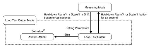
\*1. Hold down Alarm/↓ or Scale/↑ button for ≥1 second to return to the measuring mode while setting parameters.
