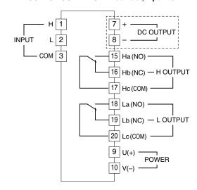
Note: The section enclosed by broken line is only with DC output option.
