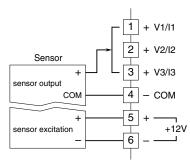
Unless the sensor output does not force minus direction such as 0 to 5 V or 4 to 20 mA, the configuration as shown below is possible. It is not available except measurement range 1 to 5 V,  $\pm 5$  V, 4 to 20 mA or 0 to 20 mA.
