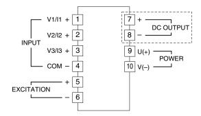
Note: The section enclosed by broken line is only with DC output option.
